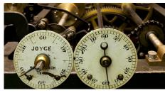
The clock was also designed by Lord Grimthorpe and built by J B Joyce and Co of Whitchurch in 1869. It is a "flat-bed" design comprising three "trains". The left-hand train operates the hour bell's chimes
