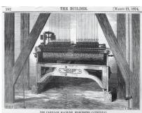
and Bland and played tunes on fourteen of the fifteen bells. It is a large "musical box" using pinned drums to activate mechanical hammers on the bells. There are seven barrels each comprising seven tunes which are a mixture of Victorian folk tunes and hymns.
