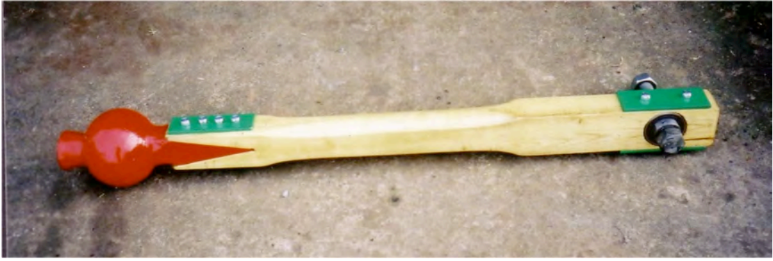
Fig.3. Two-piece tenor clapper for St Philip & St James, Hallow, Worcs.
