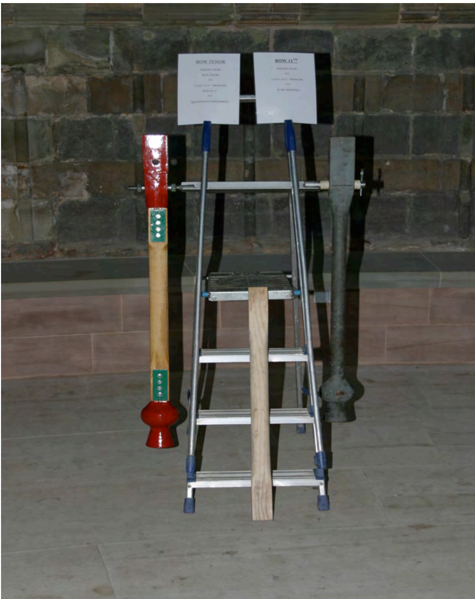
Fig.4. Bow tenor clapper and new shaft for 11 th bell shown next to unmodified unit.
