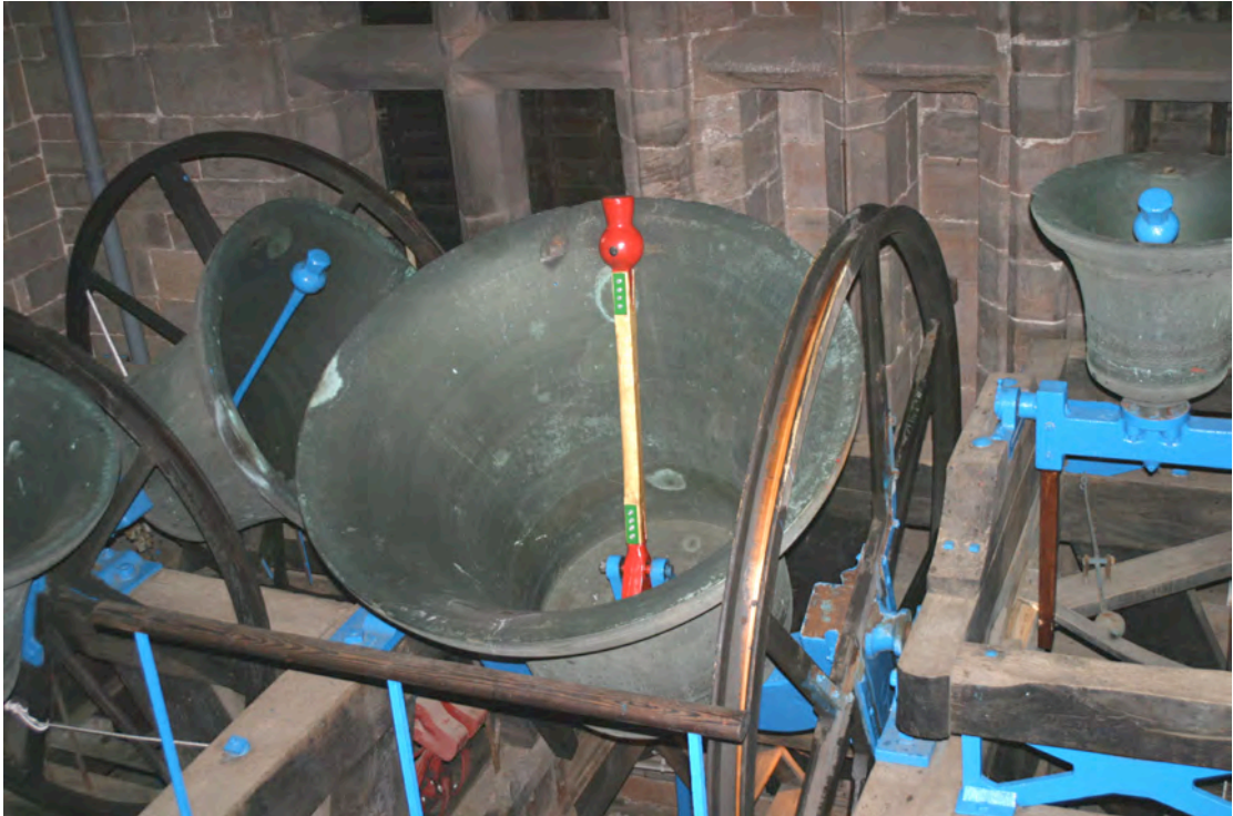
Fig.1. Worcester Cathedral tenor bell fitted with three-part composite clapper.
