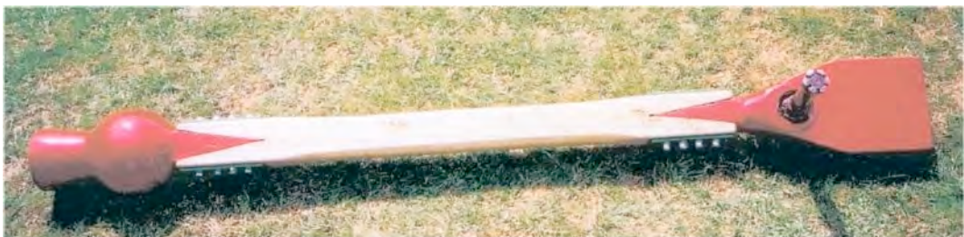
Fig.2 Three piece "Worcester Clapper" showing detail of joints and gudgeon pin bearings.
