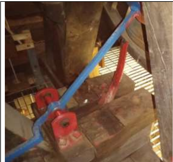
7 th clock hammer (mounting in 6 th pit)
