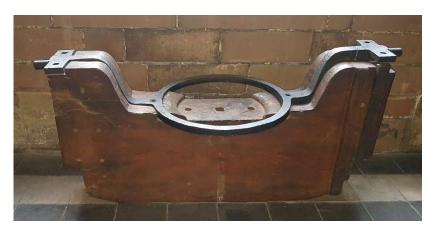
The gudgeons would rotate in gun metal bearings on the top of the bellframe. The bell would swing on these bearings, rotating 360 degrees clockwise and anti-clockwise so the bell could be rung in the traditional English style.
