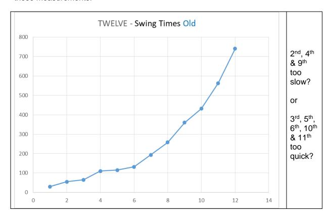
Ideally this should be a smooth line – it is clear that adjustments were required. One way of viewing this is to see the  $4^{th}$  and  $9^{th}$  bells and to a lesser degree, the  $2^{nd}$ , as too slow. But as it is close to impossible to speed bells up (at least not without rehanging) the other way to perceive the line is that the key fixed points are the  $4^{th}$ ,  $7^{th}$ ,  $8^{th}$ ,  $9^{th}$  and tenor, meaning that other bells should be <u>slowed down</u>.
